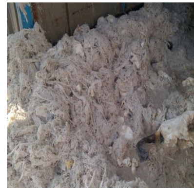
Improperly Slushed poly sheets
